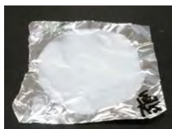
Fig. 3 Wood-Derived CNF Applied to and Dried on Aluminum Foil
