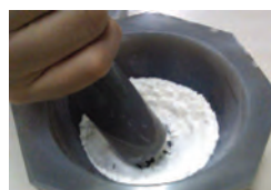
Fig. 2 Homogenization by Pulverizing
