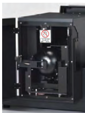
Fig. 3 Inside the ISR-1503 (left) and with Sample Installed (right)
