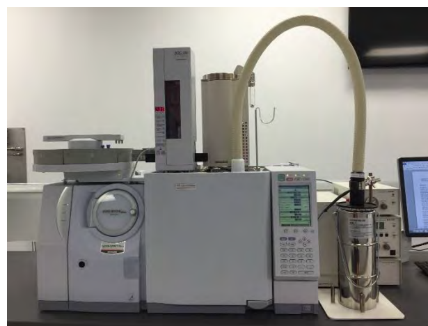
Figure 1: Frontier Multi-Shot EGA/PY-3030D pyrolyzer and AS-1020E Auto-Shot sampler installed on the Shimadzu GCMS-QP2010 Ultra
