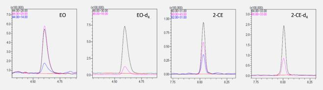
Figure 3. Chromatograms of EO, 2-CE, EO-d<sub>4</sub> and 2-CE-d<sub>4</sub> (standard 50 ng/mL)
