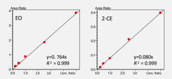
Figure 2. Calibration curves for EO and 2-CE
