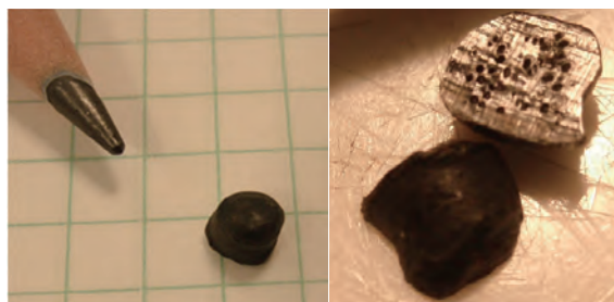
Fig. 1 (Left) Approx. 5-mm Diameter Plastic Pellet (Right) Cross Section
