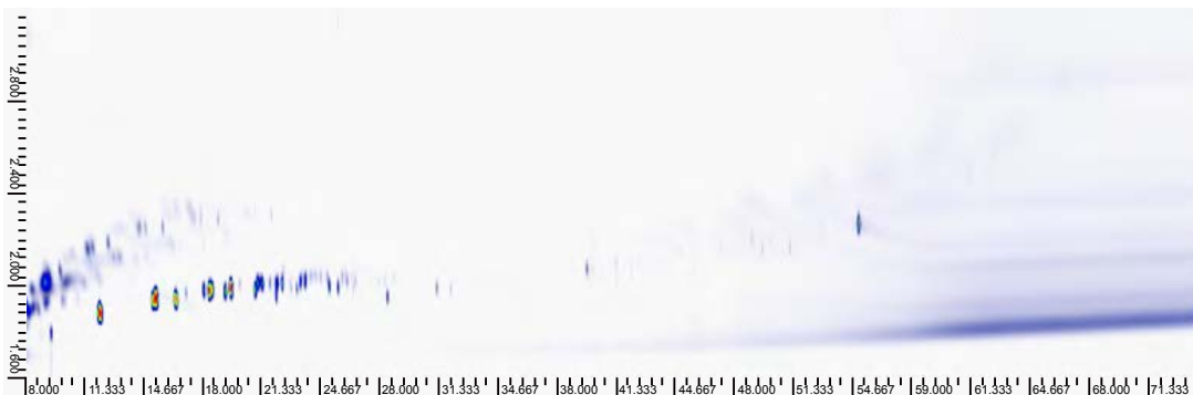
Figure 1: Comprehensive GCXGC-qMS total ion chromatogram of gasoline. X-axis: First dimension, retention time in seconds. Separation based on polarity. Y-axis: Second dimension, volatility-base separation in seconds.
