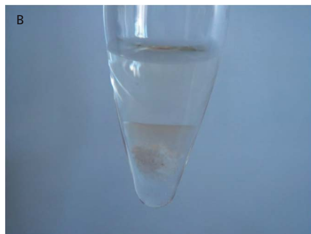
Figure 2: influence of QuEChERS salts on urine extraction/partitioning: A: acetonitrile with urine sample lead to one phase / B: acetonitrile, QuEChERS salts and urine lead to 2 phases.
