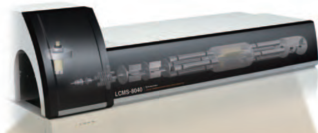
Improved ion optics of the LCMS-8040 for Ultra fast scan speed with enhanced sensitivity
