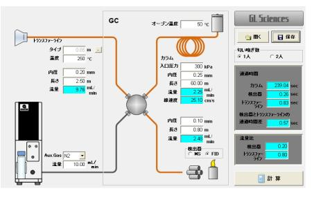
Bifurcate the exit of the GC column inside the GC oven, carrying gas to the detector such as FID or MS, and simultaneously to the operator side (nose) on the other side.
