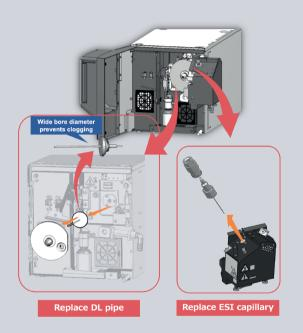
Removal and installation can be performed without tools and without breaking the vacuum.
