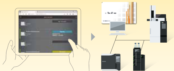
Directly access a GC unit in the laboratory from a smartphone or tablet computer
