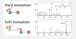
CI is a softer ionization method than EI. Fragmentation is less likely to occur, so molecular weight information is more readily obtained. Negative chemical ionization (NCI) or negative ion chemical ionization (NICI) enables selectively measuring, with ultra-high sensitivity, chemical substances with an electron affinity, such as chlorine-based compounds.
