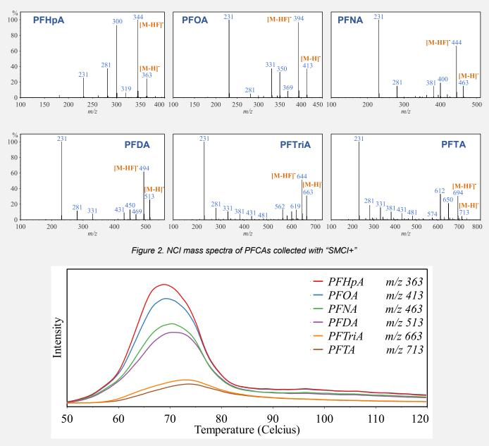
Figure 3. EIT profiles of [M-H]<sup>-</sup> ions from NCI mode of "SMCI+" for PFCAs
