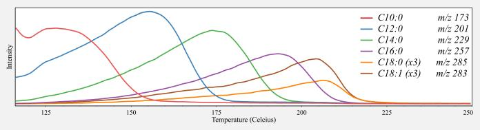
Figure 3. EIT profiles of QCI mode for a mixture of FFAs
