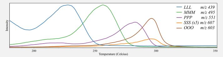
Figure 5. EIT profiles of SMCI mode for a mixture of TGs
