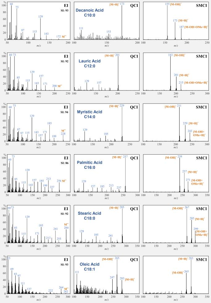
Figure 2. EI, QCI, and SMCI mass spectra of FFAs collected with "Smart IS+" and "SMCI+". SI: Library similarity index
