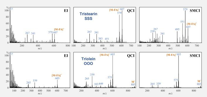
Figure 4. EI, QCI, and SMCI mass spectra of TGs collected with "Smart IS+" and "SMCI+". The formula of FA refers to C<sub>12</sub>H<sub>24</sub>O<sub>2</sub> for LLL, C<sub>14</sub>H<sub>28</sub>O<sub>2</sub> for MMM, C<sub>16</sub>H<sub>32</sub>O<sub>2</sub> for PPP, C<sub>18</sub>H<sub>36</sub>O<sub>2</sub> for SSS, and C<sub>18</sub>H<sub>34</sub>O<sub>2</sub> for OOO
