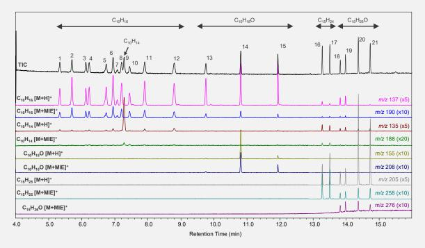
Figure 3. Total ion chromatogram of the terpene mixture. Extracted ion chromatograms for the  $[M+H]^+$ ,  $[M+H-H_2O]^+$  and  $[M+MIE]^+$  ions of the terpenes. The elution order of the terpenes is according to the numbering indicated in Figure 1.
