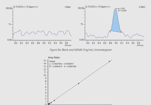
0 10 20 30 40 50 60 70 80 90 100 Conc.Ratio (ppb) Figure 9b: Calibration curve for NDMA 1-100 ng/mL
