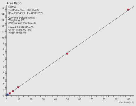
Figure 8: Calibration curve of NDMA
