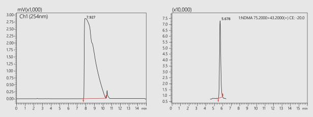
Figure 7: UV Chromatogram of Ranitidine (left) and MS chromatograms of NDMA (right) show complete chromatographic separation of API and impurities.
