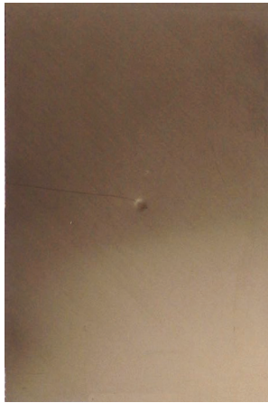
Fig. 3 Specimen After Impact Test (30.5 J Impact Energy)
