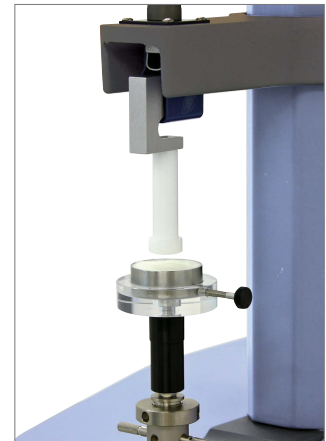
Load cell attached to crosshead
