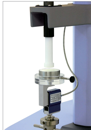
Load cell attached to lower jig
