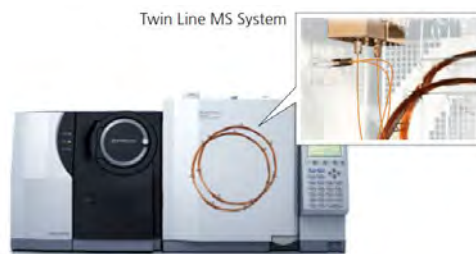
Fig. 1: GCMS-TQ8040 with Twin Line MS System
