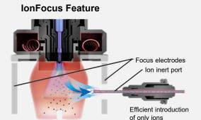
Removal of neutral particles (matrix) that causes matrix effects and contamination
