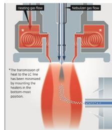
Figure 3. Heated ESI probe
