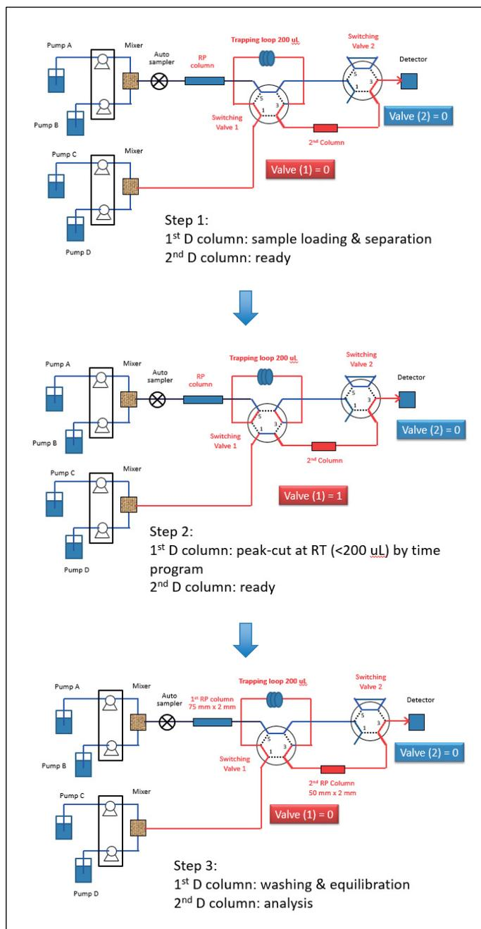
Figure 2: Schematic diagram of 2D-LC/MS/MS and operation scheme
