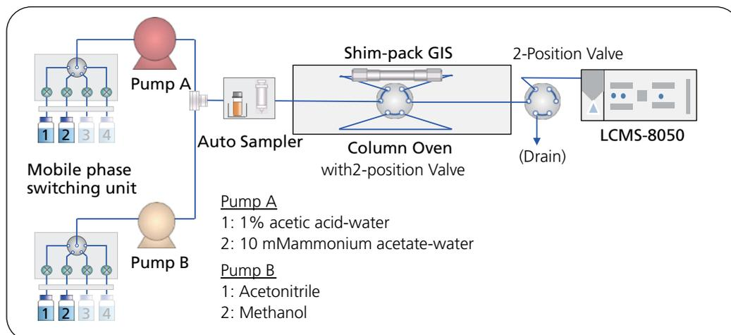
Figure 1 Nexera X2 UHPLC system with mobile phase switching unit
