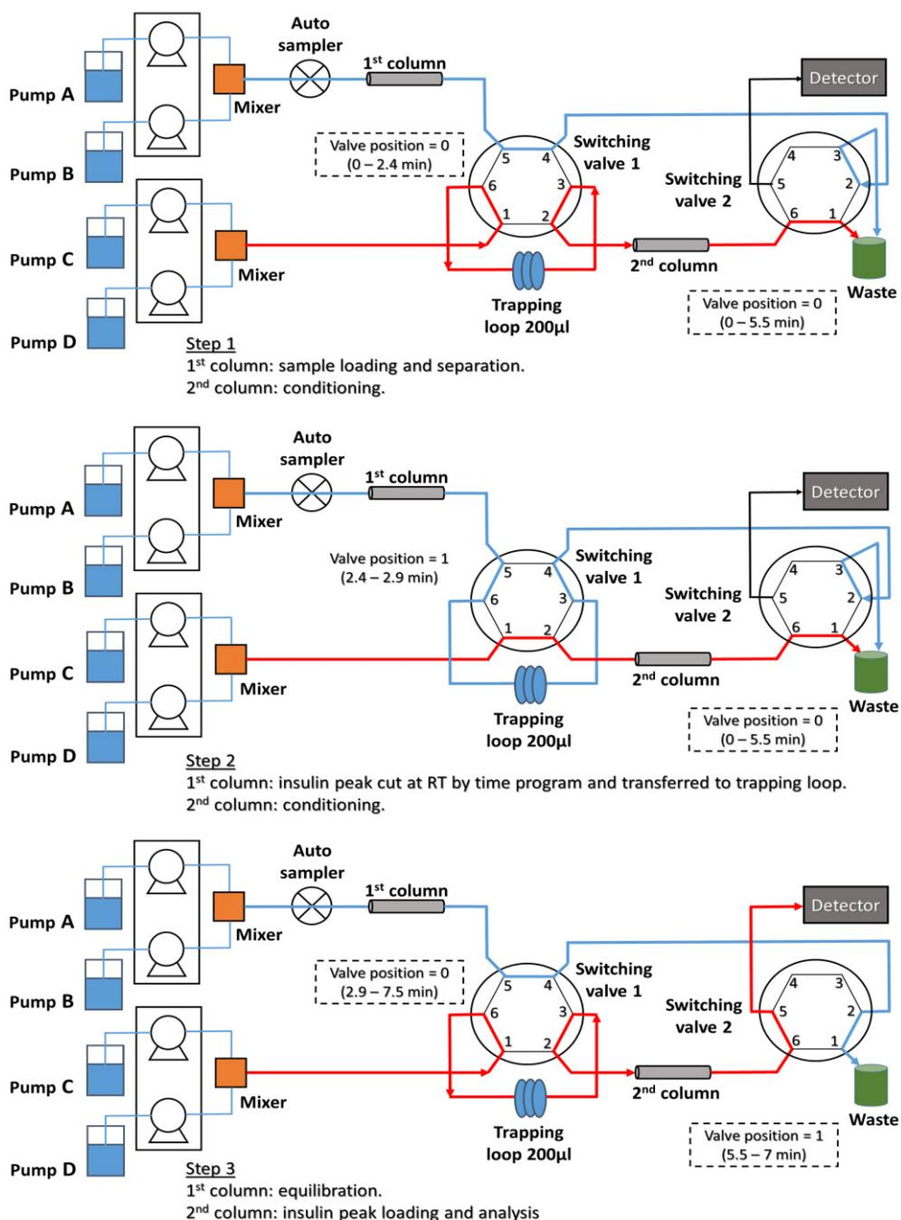
Figure 1. Multi-dimensional LC-MS/MS schematic diagram and operation scheme
