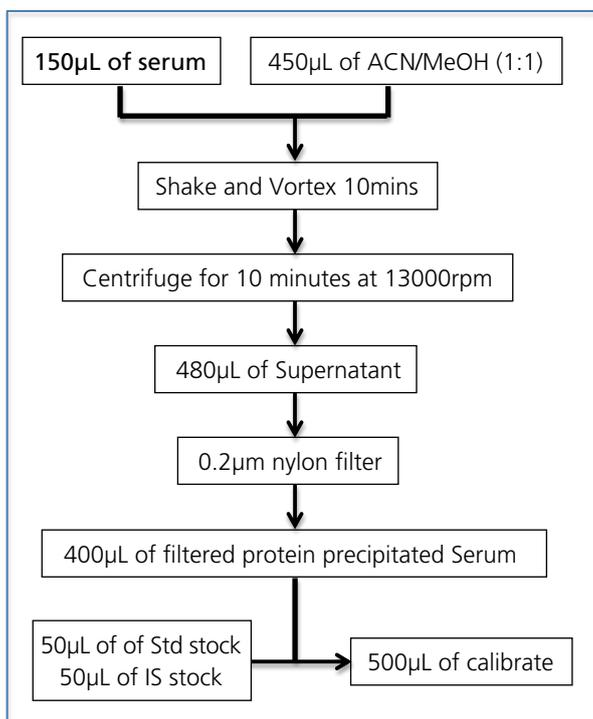
Figure 1: Flow chart of serum sample pre-treatment method
