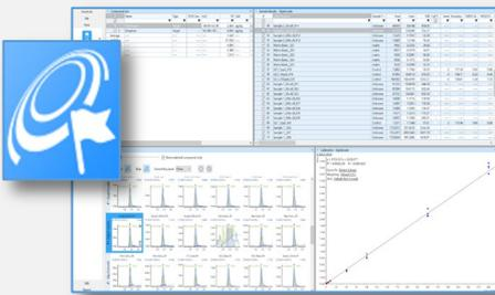
Mass spectrometry laboratories can acquire thousands of chromatograms per day. LabSolutions Insight provides tools to streamline data review and focus on the chromatograms that need critical attention. It also automatically applies your peak detection criteria to data and flags any deviations, allowing you to analyze data more efficiently.
