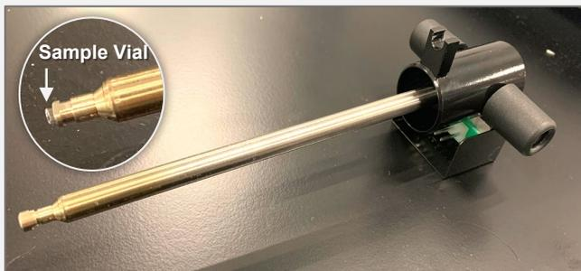
The DI unit enables samples to be injected directly into the ion source without passing through the gas chromatograph. The DI probe can be heated up to 500°C under vacuum conditions. As a result, mass spectra of high polarity and high boiling point compounds can be generated easily. The analysis is performed by simply placing the sample in a sample vial that is secured in the DI probe.
