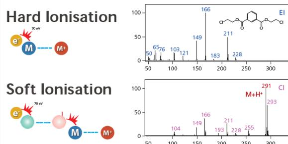
CI is a softer ionization method than EI. Fragmentation is less likely to occur, so molecular weight information is more readily obtained. Negative chemical ionization (NCI) or negative ion chemical ionization (NICI) enables selectively measuring, with ultra-high sensitivity, chemical substances with an electron affinity, such as chlorine-based compounds.
