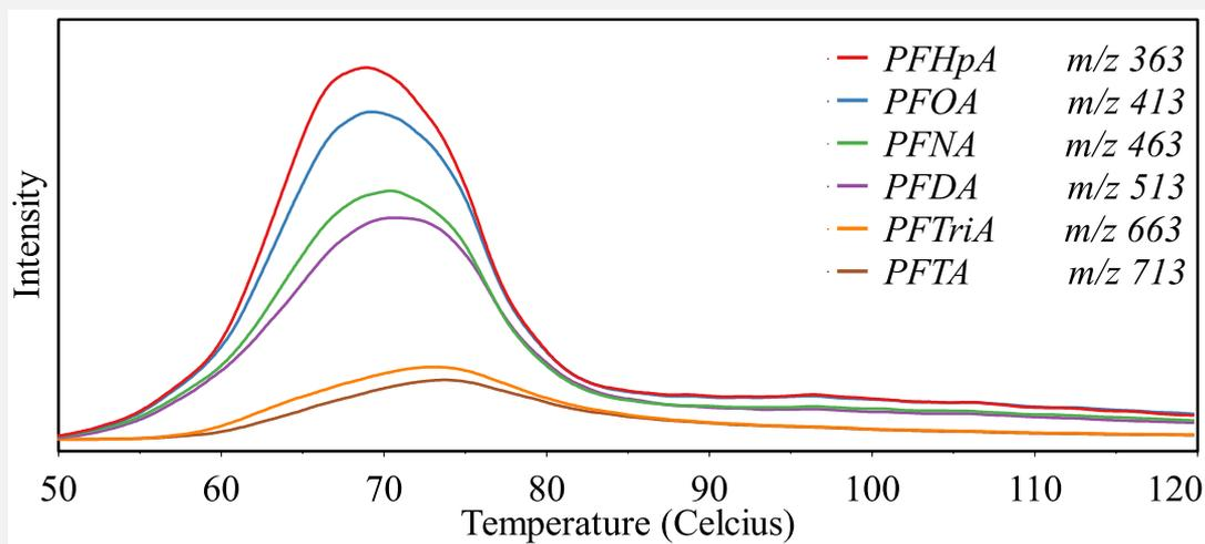
Figure 3. EIT profiles of  $[M-H]^-$  ions from NCI mode of "SMCI+" for PFCAs
