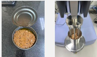
Texture evaluation of tuna flakes using EZ Test
